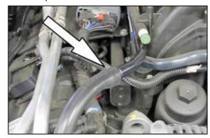
32. Connect the open end of the crank case vent hose to the factory crank case vent tube as shown.
