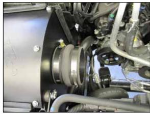
23. Install the provided hump hose (08699) onto the filter adapter and secure with the provided hose clamp.
