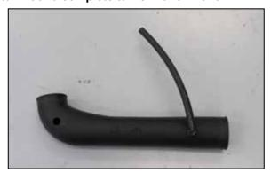
26. Install the provided crank case vent hose onto the fitting as shown.
