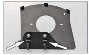
12. Install the two heat shield bracket assemblies onto the heat shield as shown.
