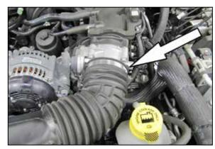
5. Loosen the hose clamp securing the factory intake tube to the throttle body.
