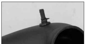
28.Install the provided grommet and factory inlet air temperature sensor into the K&N® intake tube as shown.
