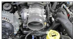
24. Install the provided silicone hose (08690) onto the throttle body and secure with the provided hose clamp.
