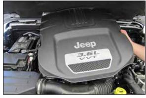
2. Lift up and remove the engine cover.
